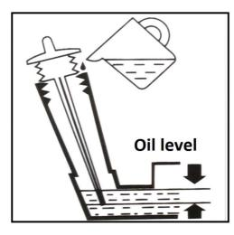
Fill the engine with the correct amount and type of engine oil. For engine oil specifications, see below.
