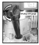
The engine **MUST** be filled with the correct amount of engine oil supplied with the delivery before its first commissioning. The bottle with engine oil <u>may contain larger amount</u> than required for the particular engine type. For specifics refer to the Technical data section.
