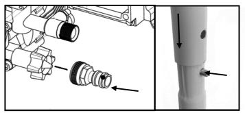
The low-pressure inlet on the pump must be fitted with the garden hose adaptor, included in the delivery.
