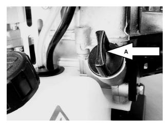
It's advisable to replace the engine oil after using the device (according to the maintenance schedule). Turn the engine off. Allow the device to cool slightly to keep the temperature below 50 °C. This prevents possible burns. It's advisable that the engine is still warm. Warm oil flows out of the engine much easier.
